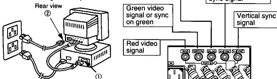
① Connect the BNC singal cable (Not supplied) to the monitor's port.
