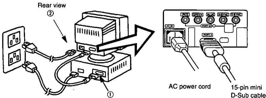
① Connect the supplied signal cable to the monitor's port.
